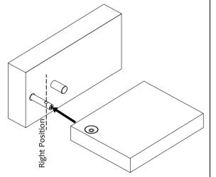
In each hole in the second piece, put in a cone shaped safety screw and tighten with a cross (philipps) screw driver - without forcing. The 2 parts will now be safely attached.
